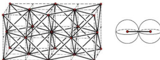
FIGURE 5. The face-centered cubic lattice
