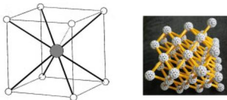
FIGURE 8. The body-centered cubic lattice
